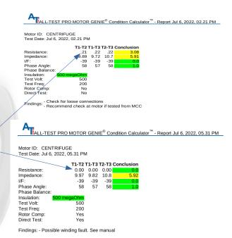
I^2R 75 Rated Amps 0.22 Resistance 3712 Watts estimate 60% Loss 2227 Watts
