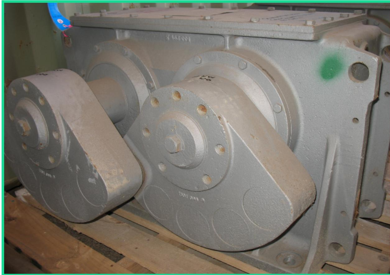
Image of an Exciter Gearbox from a vibrating screen
